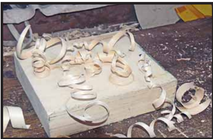
Figure 1b (below). Curley chips from air dried wood.
