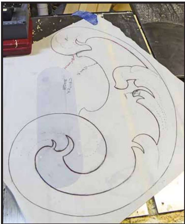
Figure 3 (above). Refined drawing for a Wurlitzer 165. Notice the scroll is the top layer and the larger piece is beneath.
