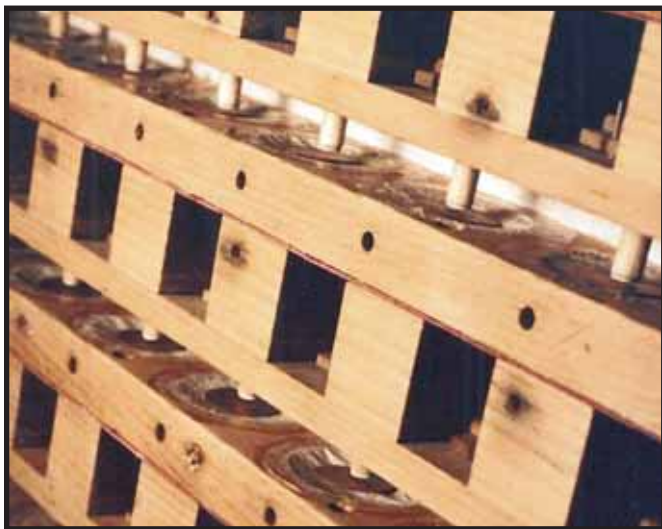
Figure 23 The pneumatic stack with new zephyr skin pouches.
