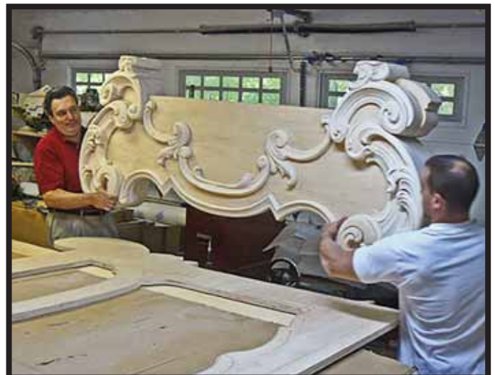
Figure 14. Center bottom section for a Wurlitzer 165, approximately 16" deep at the bottom and 12" deep at the top.
