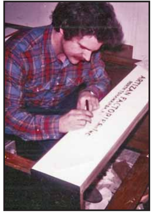
Figure 16. Mike carefully outlining the gold lettering with a black border.
