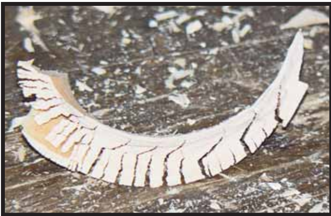
Figure 1a (above). Broken chip from kiln dried brittle wood.
