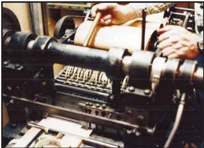
Figure 4. The B.A.B. Acme Perforator. The heavy paper master roll is at the top of the photo.
