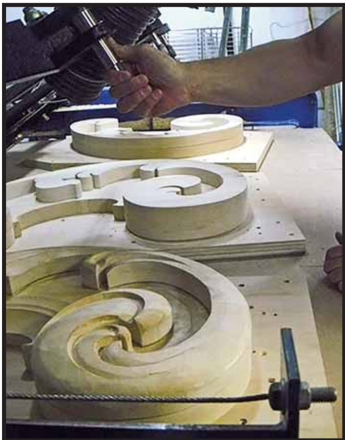
Figure 7 (top left). The sawn piece carved to the pattern. Figure 8a (middle left). The glued up pieces on the duplicator. Figure 8b (bottom left). Closeup of the original next to each band sawn piece. Figure 9 (top right). Examples of chisels. Figure 10 (middle right). The rough-outs right off of the machine. Figure 11a (bottom right). Refining the rough-outs.
