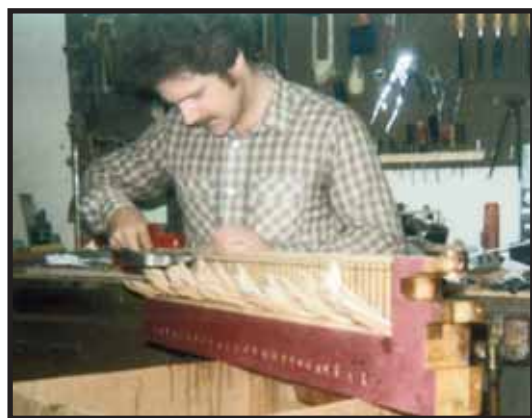
Figure 19. Mike inspects the restored pallets.
