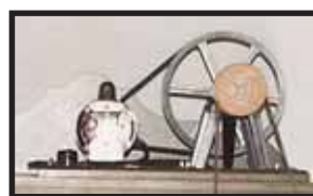
Figure 22. The new motor and jackshaft assembly.
