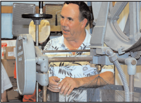
Terry Haughwout explaining the weaving machine that is used to make new wiring harness' for restoring the Mills Violino.
