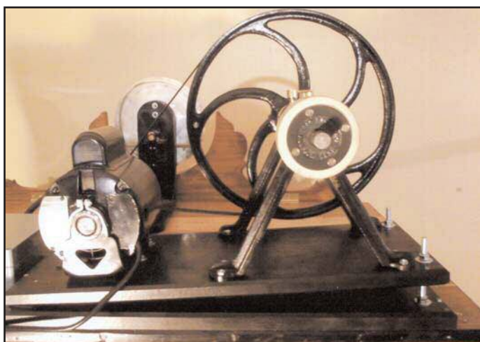
Figure 6. The motor and countershaft assembly sits on top of the organ.
