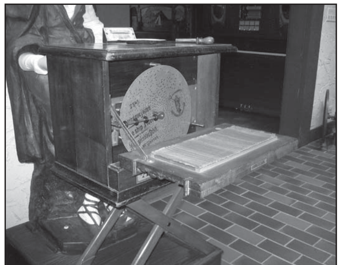
Figure 4. Opening the case of the “Savoyard” reveals the single disc-playing mechanism.
