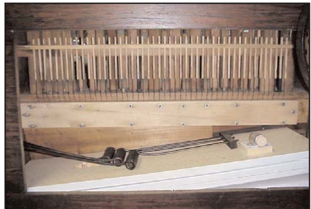
Figure 8. The push rods going into the wind chest. The pneumatics on the valve chest will push on these to play the organ.
