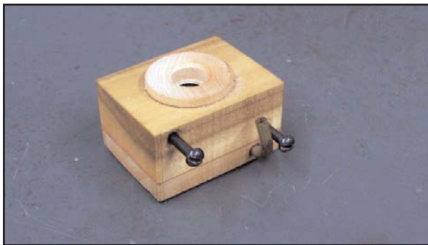
Figure 4 (top). The bottom section of the block valve with the pouch and bleed.
