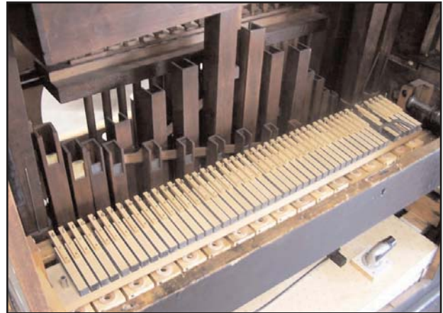
Figure 7. The newly fabricated valve chest and pneumatics mounted in the organ. The tips on the pneumatic fingers are positioned over the tops of the push rods.
