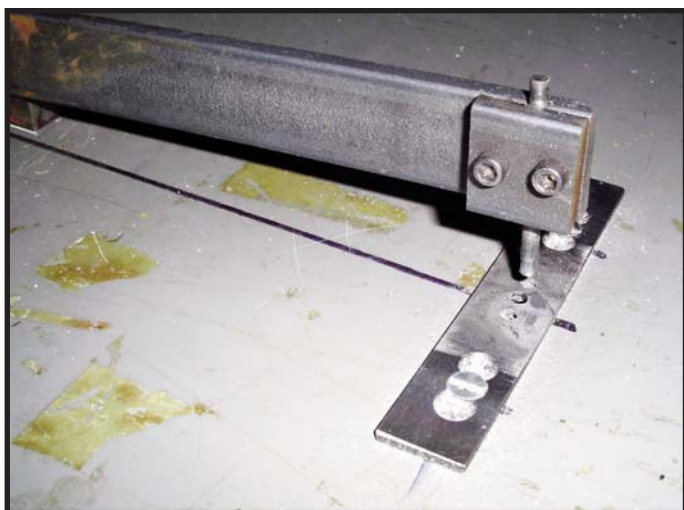
Figure 4. This shows the punch and die assembly. The punch is made from rod by lathe-turning a taper of about three degrees near both ends, making it reversible. Each die plate has a series of nine holes, allowing shifting between three positions as the holes dull. The attachment holes in the table surface are over sized. The punch is brought into the hole to set the plate's location, then the screws are tightened to lock it in place. Both parts were made from oil-tempering steel, heated until red hot, and dropped into waste motor oil.
