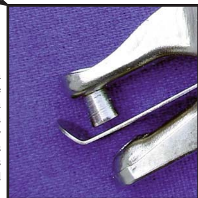
Figure 5. This photo of a cheap hand-punch shows the conical shape desired on a swinging arm. On such a design the punch actually rotates as it enters and leaves the die, and the taper allows both smooth motion and reduced clearance.
