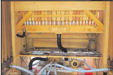
Figure 9 (above) reveals an over-all view of the back of Clark's Organ. The computer is located in front of the large open flute pipes.
