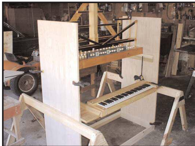
Figure 3. The case shell, showing early placement of components. Note the sides of unfinished oak plywood.
