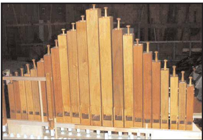
Figure 2. The row of stopped flutes, complete and installed on the organ chest.
