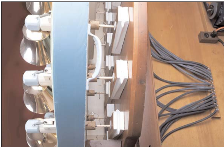
Figure 2. A top view looking down on the bronze bells on the façade with corresponding backboard with mounted pneumatic and valve chest.
