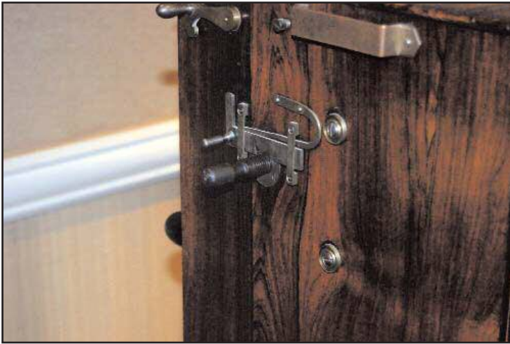
Figure 6. A view of the left side of the case reveals the barrel-changing mechanism and keyframe lift.
