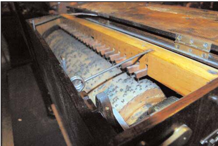
Figure 7. The pinned barrel and original key frame are seen in this photo. Note the pristine condition of the organ.
