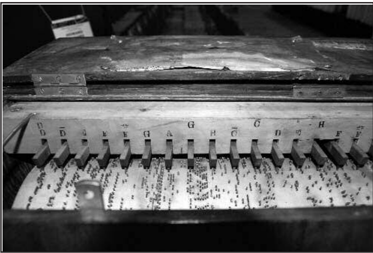
Figure 10. The deKleist's key frame and pinned barrel.
