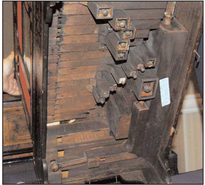
Figure 8. A view under the organ reveals many stopped and mitered pipes.
