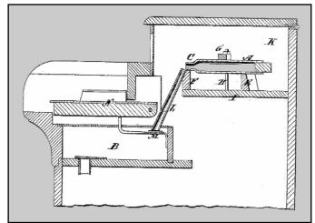
Figure 10. William Standing's patent #128,566 (7/2/1872). The typical keyboard (N) is depressed allowing for the valve facing (M) to move away from the air supply tube (L). Air under pressure then goes from the reservoir (B) to the mouth of the glass tubes (C) and provides a musical sound.
