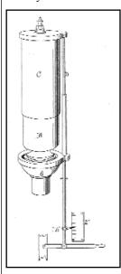
Figure 1. Otto Kromer's patent #142,166 reveals the bell (B) covered by another bell (C), which is telescoped over the inner bell (B). The overlying bell (C) is controlled by a rod (D), which attached to an index (E), set to any of the letters of the musical scale.
