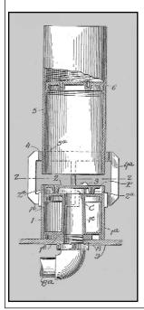
This invention is a novel improvement in whistles for musical instruments, such as calliopes. The object of the present invention is to insure more direct and uniform pressure of the air discharged from the cup of the whistle; and to improve the construction of the air distributing devices in the cup of the whistle.
