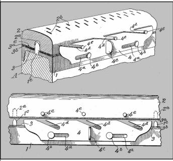
Figure 27. Norman Baker's patent #1,619,690, "Tracker Bar," was granted March 1, 1927. The tracker bar can be seen to be constructed in two pieces (2) and (1) with a screen (3) between. Attachment of the top portion to the bottom is accomplished via the sliding cam (4), which attaches via slots (4a) over protruding pins (4b).
