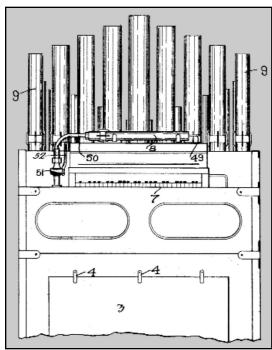
Figure 15. Joseph Ori's 'Pneumatic Calliope" patented September 5, 1916. This is patent #1,197,302 and features not only the 43-note calliope which was to become the standard for air calliopes but also the unusual "special variable pitch whistle" (8) discussed in the text of this article. See Figure 20 for another view of this whistle.
