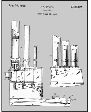
Figure 29. Joseph Sylvia's "Calliope" which was patented on August 29, 1929 and numbered #1,725,025. Examination of this patent drawing reveals the simplistic method of playing a whistle (7) by cords (22) and pulleys (25 & 26), the cords being attached to keys (17) on the keyboard (16).
