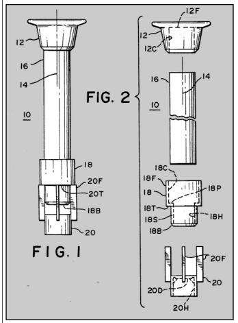
Figure 30. Patent #5,255,589 details a normal and exploded view of Caulkin's "Calliope Pipe Converter."
