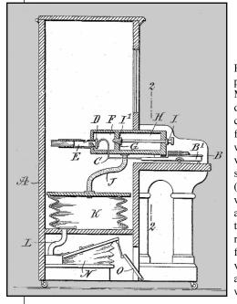
Figure 12. Mr. Earley's patent, #847,169 dated March 12th, 1907 depicted an uprightcased machine with a foot pump bellows (N) which supplied a reservoir (K) which in turn supplied a wind chest (H) of which various whistles (E) were attached. Depressing the key (B) caused the rod (C) to pull away from the opening, or (D) which valve, allowed any particular whistle to sound.
