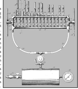
Interestingly enough his varying the strength of tones involves reducing the high pressure in the tank (19) noted in Figure 21 by way of a reducing valve (23). In the patent he states:
