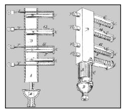
Figure 2. Otto Kromer's second patent, #141,280, details a whistle with multiple valves (E). F are the valve stems which are held open by springs (J). When the valve stems are pulled, the valve (E) is pulled to close off the whistle bell and "play" a particular note.
