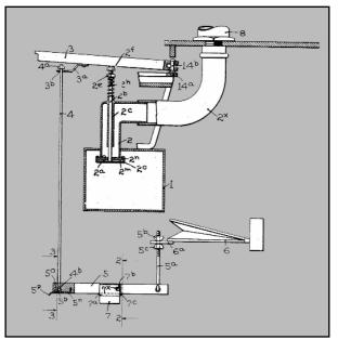
Figure 24. Norman Baker's patent #1,512,666 describes the interrelations of manual (top of drawing) and automatic (bottom of drawing) playing of the air whistle (8). Besides this relationship the patent notes the easy cessation of automatic playing (to stop ciphers of particular notes) by disconnecting the connecting rod (4) from the fulcrummed lever (5).
