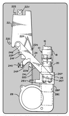
Figure 31. Caulkin's "Pneumatic Activator" is presented in patent #4,619,177. This is a valve assembly to allow the pipe to play.
