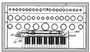
Figure 16. This is an overhead view of Ori's invention, showing placement of the keyboard, the variable pitch whistle (8) and the individual whistle locations (9). The pressure gauge is located in the middle of the top row of whistles, facing away from the operator! A strange location, to say the least.
