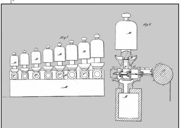
Figure 5. Joshua C. Stoddard's patent #13,668 for his "Musical Instrument." Figure 1 shows the line up of eight steam whistles (B) on the manifold (A). Figure 2 is a cross drawing of the puppet valve showing the end of the valve steam being activated but studs on the pinned barrel (D). It is this activation that opens up the valve and lets steam go from the manifold (A) through the base of the whistle (G).
