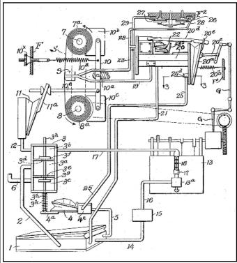
Figure 25. Baker's patent #1,609,102 was granted on November 30, 1926 and is entitled "Vacuum Brake Apparatus." While not specific for the calliope the concept of his braking ideas encompasses several mechanical musical instruments.
