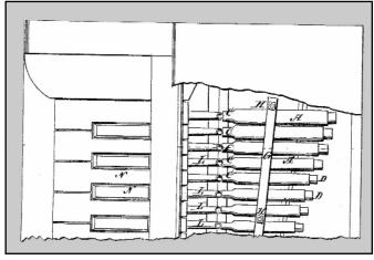
Figure 11. An overhead view of Standing's patent #128,566 shows the piano keyboard (N) and the air supply tubes (L) and the glass sounding tubes (A). (D) represents the tuning plugs.
