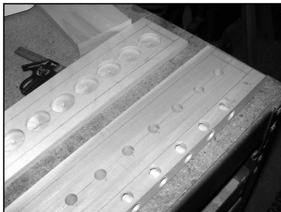
Figure 3. Drilled pouch board and main valve board.
