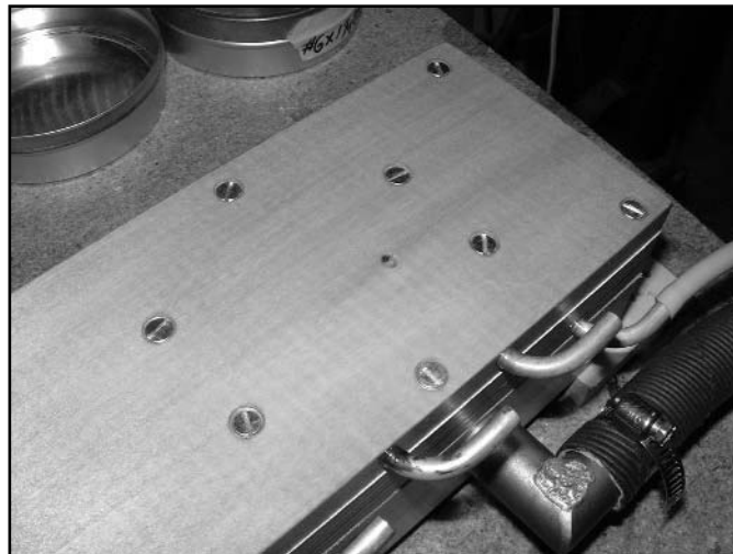
Figure 22. All layers screwed to the chest, with test vacuum supply attached.
