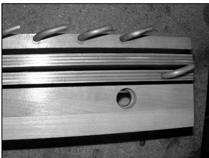
Figure 10. Elbows installed for key action and stop action.
