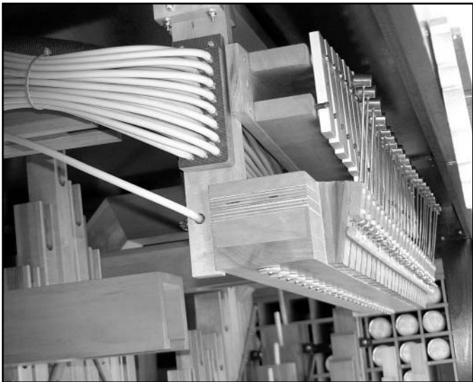
Figure 25. Position of striking pneumatics, bell bars and stop rail shown here.
