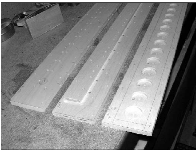
Figure 6. Port drilling completed.
