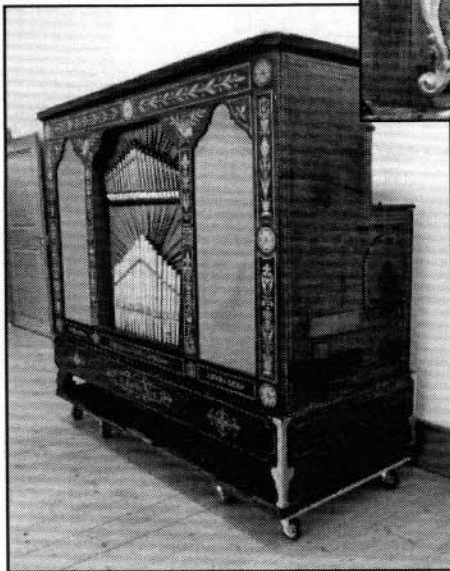
On the left is a 90 key A. Ruth barrel organ (Model 24). The organ is in the collection of the Elztalhmuseum, the museum in Waldkirch that specializes in preserving the mechanical instruments that were manufactured there.
