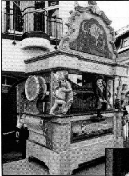
A recently-built 56 key Keller organ with exposed pipework and unusually placed drums (left). This organ uses the 56 key Limonaire scale and was built by Frederick Keller, the last apprentice of Carl Frei, Jr.
