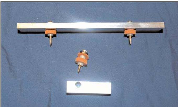
Figure 4. One of the bars showing the silicon washers. Below is the bar that was used as a tube cutting jig.
