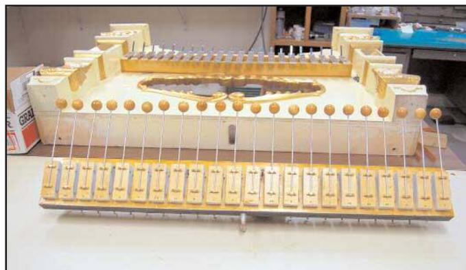
Figure 5. The striker pneumatics mounted to the chest.
