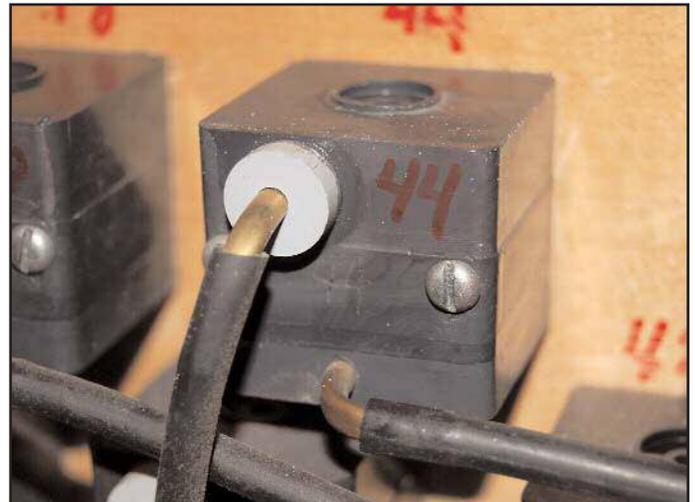
Figure 9. Valve assembly details for the tympani effect.
