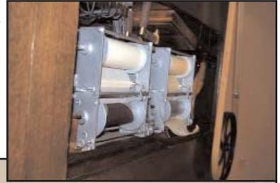
Figure 8 (right). The restored roll frames loaded with Style 165 roll music.
