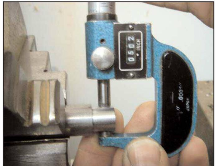
Figure 17. Measuring the shaft end.
