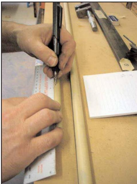
Figure 1. Marking stock for various shaft lengths.
