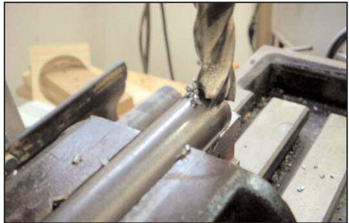
Figure 22 (above). Machining tapered square on the shaft end.
