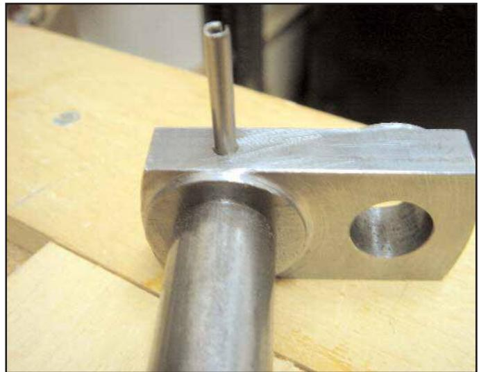
Figure 21. Installing the tension pin.
