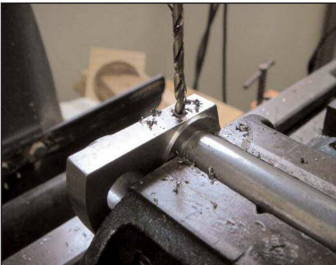
Figure 20. Drilling for a tension pin.
