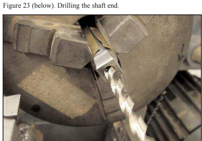
Figure 23 (below). Drilling the shaft end.
