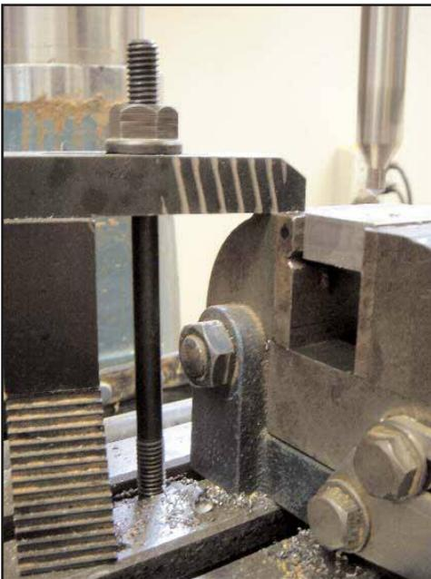
Figure 5. Center drilling.
