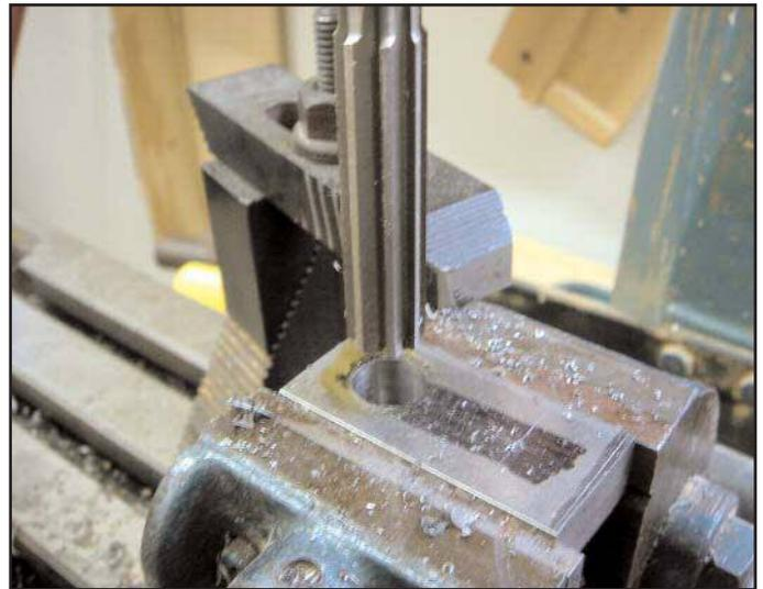
Figure 7. Reaming the drilled hole.
