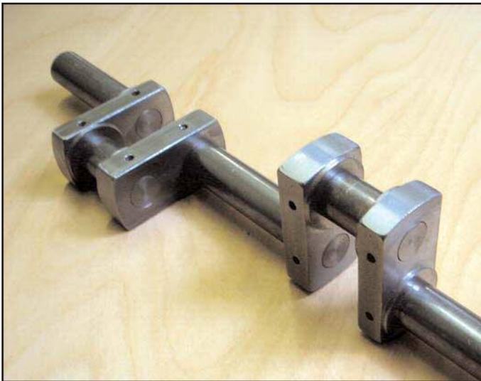
Figure 25. The completed crankshaft.
