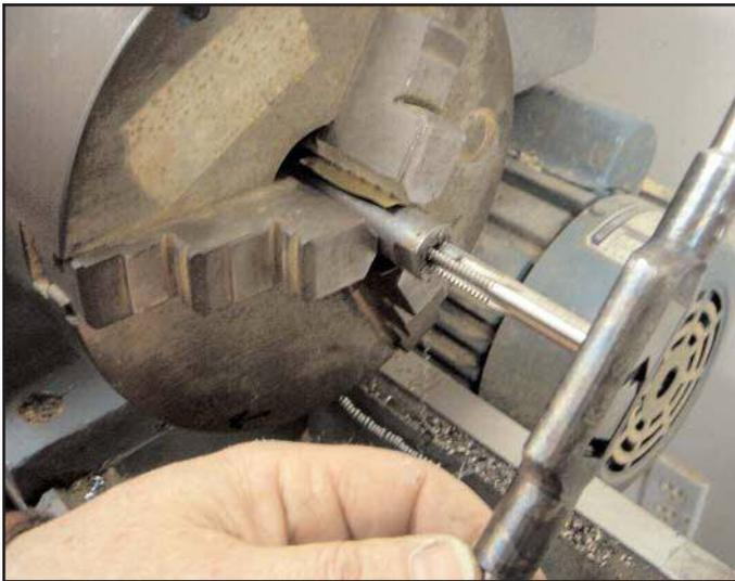
Figure 24. Tapping the shaft end.
