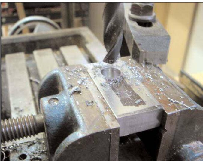
Figure 6. Drilling the crank throw.
