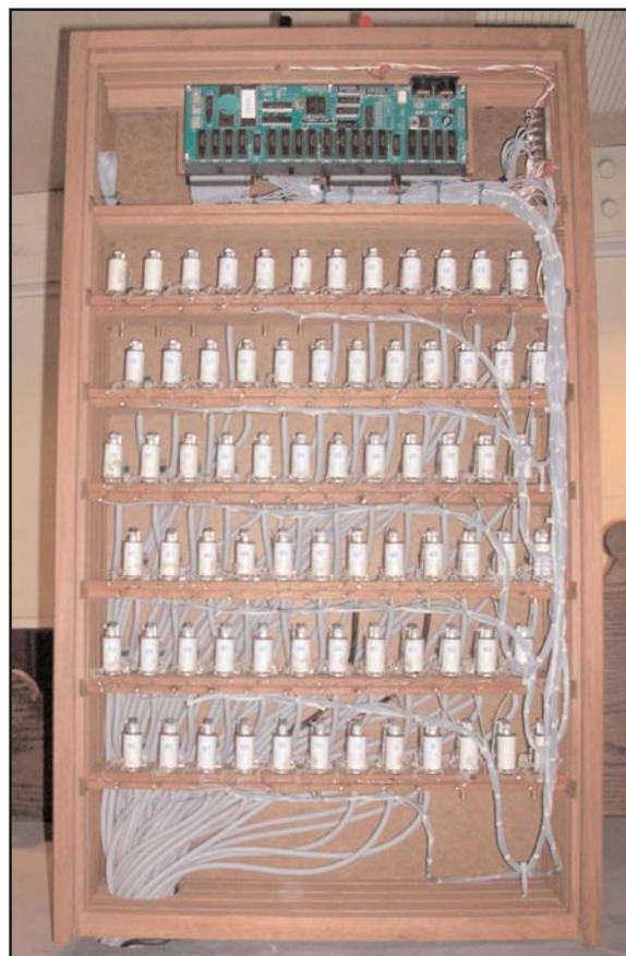
Figure 2. The box of valves for the organ.
