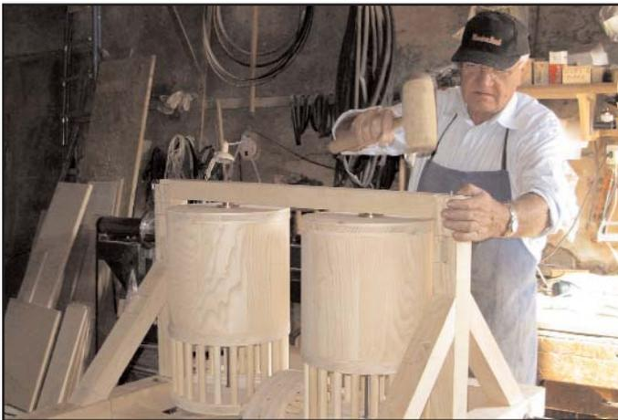
Figure 5. Mounting the barrels to the chassis.
