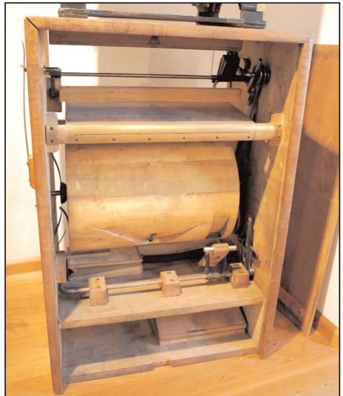
Figure 4. This Gebrüder Bruder roll player has a 100-hole tracker bar, intended to serve on different makes of organ by means of rolls incorporating the requisite scale. Author's photograph.
