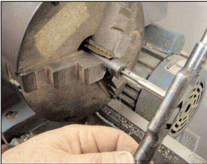
Figure 24. Tapping the shaft end.
