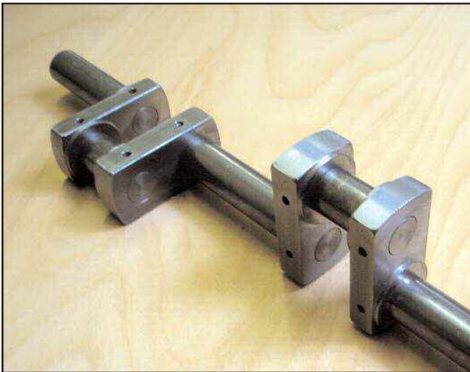
Figure 25. The completed crankshaft.
