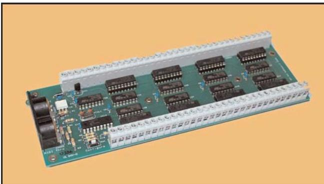
Figure 9. The MIDI driver board, with 64 outputs, controls the pipe valves in the wind chest.
