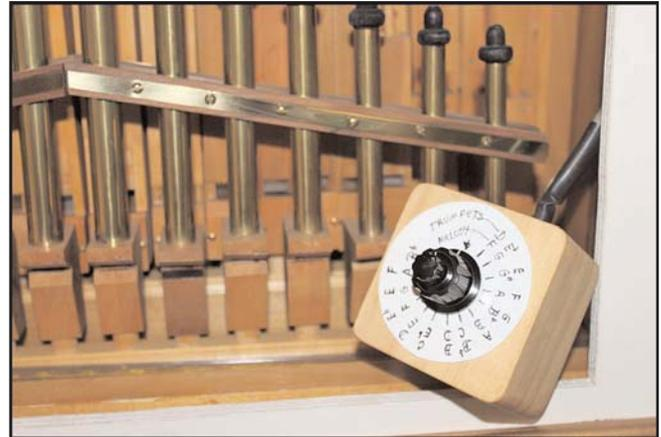
Figure 10. This “tuning box” contains a rotary switch with two decks of contacts. The larger knob turns the melody pipes “on” one at a time for tuning. The smaller knob does the same for the trumpets. The tuning box is stored inside the case when not in use.
