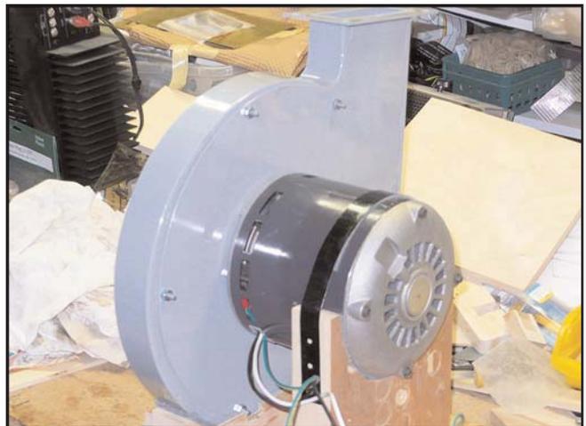
Figure 4. This blower operates on 120 VAC, and easily supplies sufficient air for a 105 type organ. It should be enclosed in an insulated box to lower noise.
