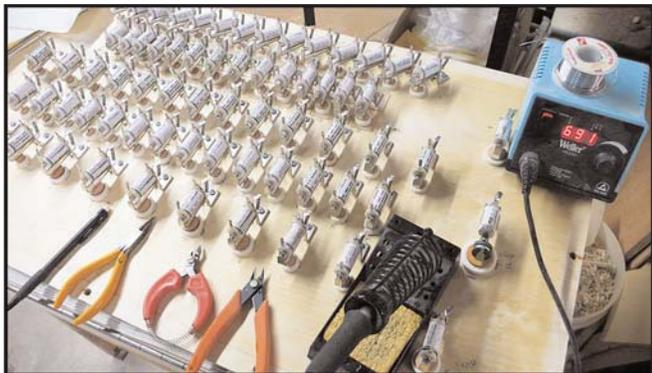
Figure 5 (above). The pipe valves are in place ready to be wired. To lessen the chance of damage to the valves, a low wattage soldering unit is used .
