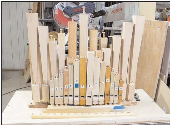
Figure 7. Melody stopped flutes, wooden trumpets, and accompaniment stopped flutes are completed and in place on the wind chest. The hinge on the front allows the lid to be raised for access to the pipe valves underneath.
