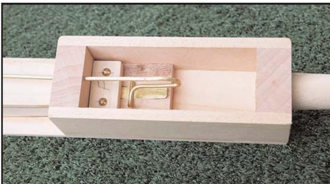
Figure 3. Visible in this photo of a wooden trumpet boot, is the brass reed that vibrates against a wood shallot. The wire is used for tuning. A wood cover attached with screws completes the unit.
