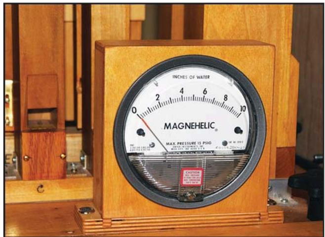
Figure 2. This type of pressure meter may be used during pipe testing, and then later installed in your organ.
