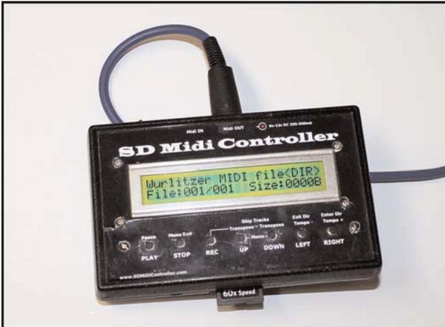
Figure 8. MIDI file player with a SD type memory card that contains over 200 band organ songs. The output of MIDI unit connects to the MIDI driver board.
