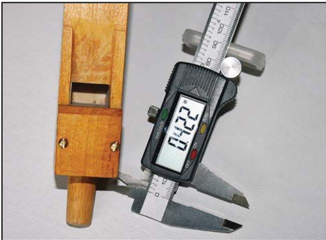
Figure 1. Electronic digital calipers with inch/metric conversion, are very useful during organ pipe construction.
