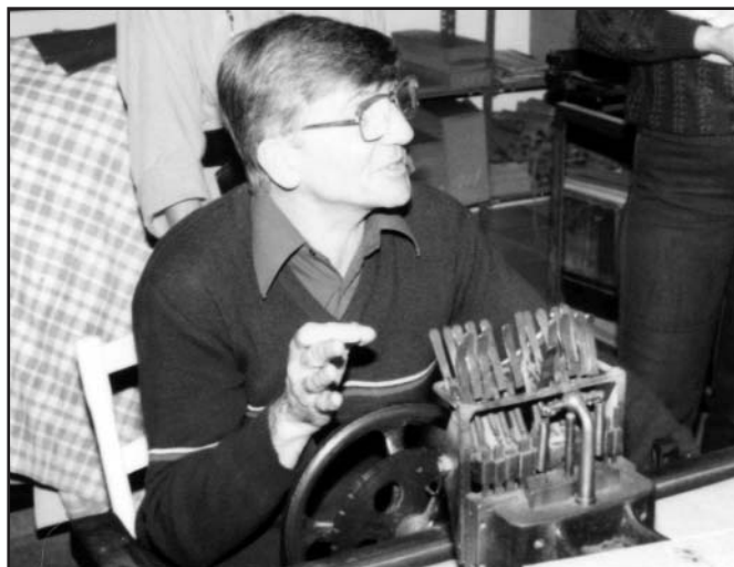
Figure 6. Detail of Arthur's unique punching machine: the head and matrix have been constructed in such a way that any size of die can be chosen with a simple click on one of the levers.
