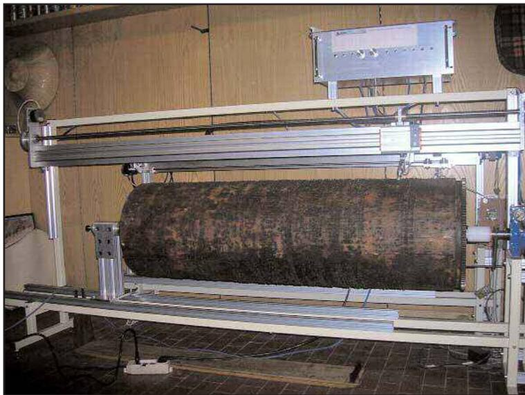
Figure 1. An overall view of the pinned barrel scanner.
