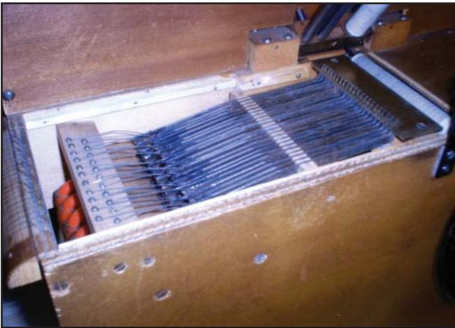
Figure 3. 22-key Perlee organ with the cover remove—you can count 22 keys.
