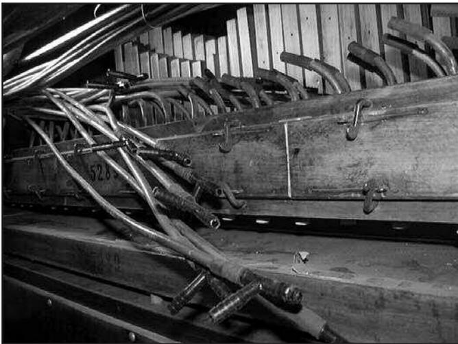
Figure 5. Another view of the Bruder valve chest showing some tees attached to the lead tubing.
