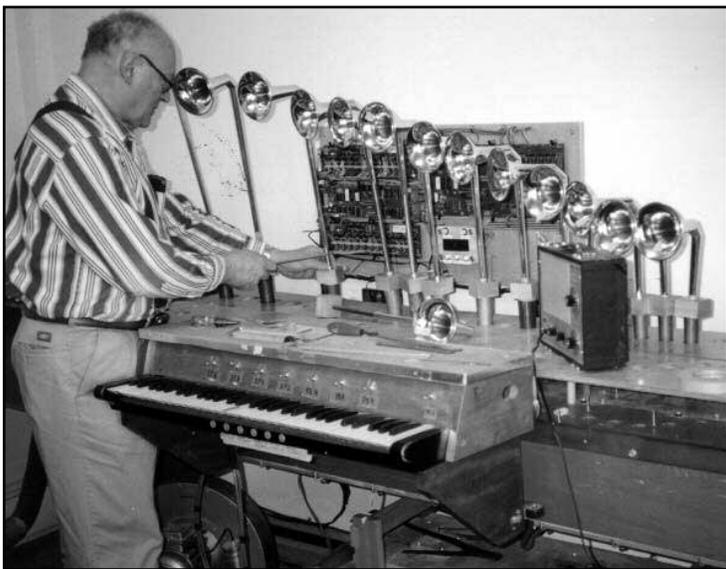
Figure 1. Lance Johnson voicing trumpets for the Johnson Style 163 band organ.
