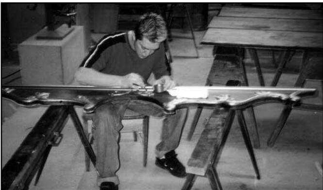
Figure 2. Skip Johnson applying gold to the Style 163 scroll.
