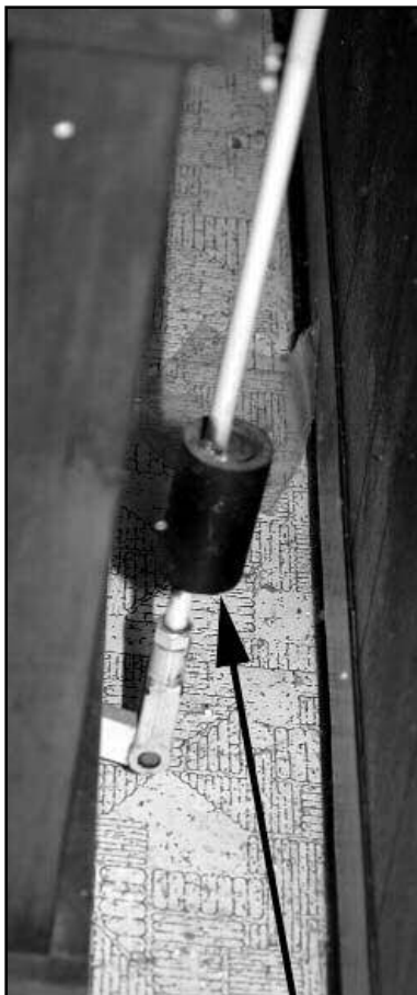
Figure 5. The arrow points to the weight placed on the vertical rod positioned in the rear of the punch. This acts as a counterbalance.
