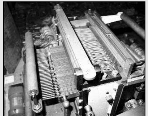
(left, above & right): The Mangels (Bruder) cardboard book duplicator. Was this made by Bruder for Mangels? It is hard to imagine the carousel company having enough use to warrant the manufacture of such a sophisticated machine. It is supposed to copy up to 80-keyless Bruder music.
