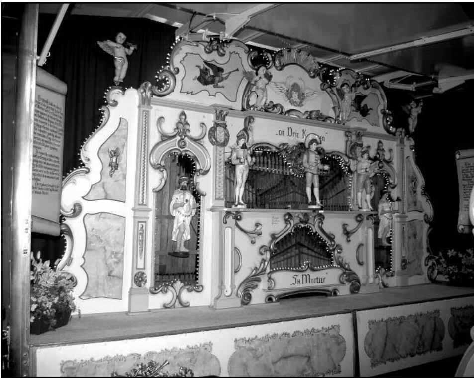
Figure 5. de Drie Kransen , an 84-key Dutch Street Organ. The organ originally was an 80-key Gavioli barrel organ but converted later to play 84-key books.
