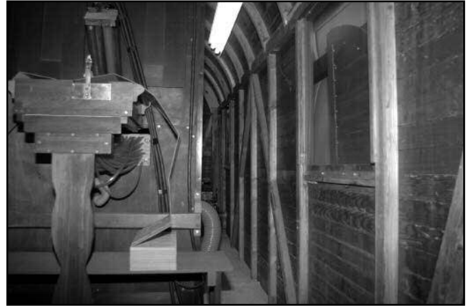
Figure 11. Inside the German-built trailer one can appreciate the wood slat sides and the curved roof.
