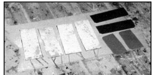
Figure 8. Shown here are all new triple-thick flap valves as well as valves for the "flip" boards (which are under spring tension).
