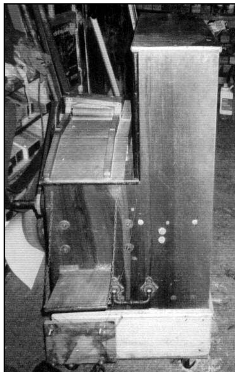
Figure 3 (left). A “before” photo of the snare side of the organ. The grease holes had no covers; the motor was mounted on the side of the case and there were corks in the snare drum holes (for air supply to the beaters).
