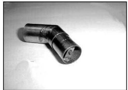
Figure 15. Air motor nipple with check valve.
