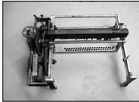
Figure 27. Roll frame removed from calliope.
