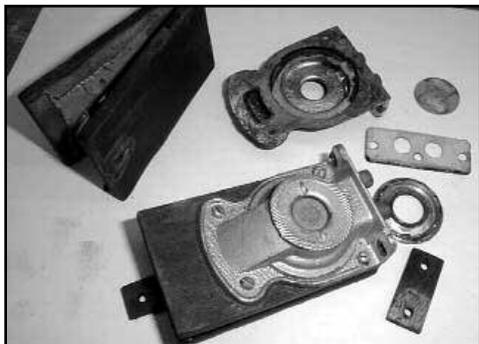
Figure 19. Pneumatic stack valve unit and disassembled parts.
