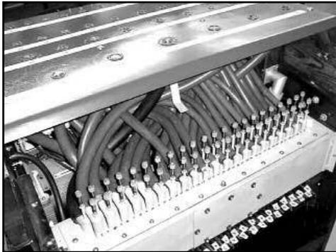
Figure 40. Hoses from windchest to pipework installed.
