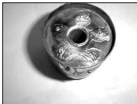
Figure 45. Failed solder joints.
