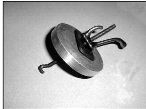
Figure 50. A tool for tuning the pipework.
