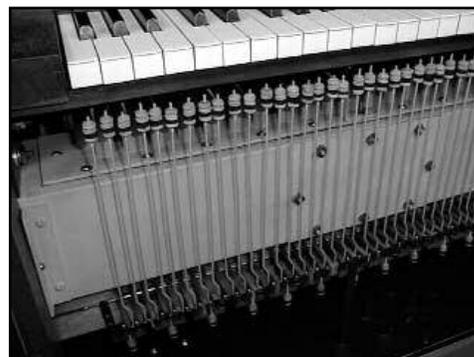
Figure 43. Windchest linkage installed.
