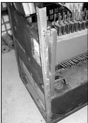
Figure 9. Bent angle iron frame member.
