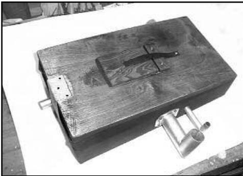
Figure 12. Restored vacuum reservoir.
