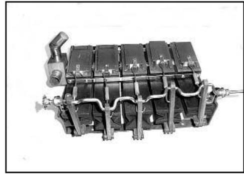
Figure 14. Restored air motor.
