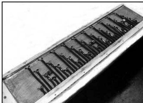
Figure 17. Inside view of the pneumatic stack.
