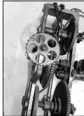
Figure 28. Closeup of roll frame gear arrangement.
