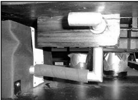
Figure 13. Restored vacuum valve to control the roll frame speed.
