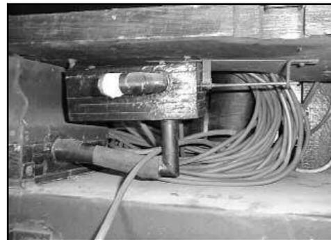
Figure 8. Unrestored vacuum valve to control the roll frame speed.
