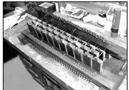
Figure 16. Unrestored pneumatic stack.
