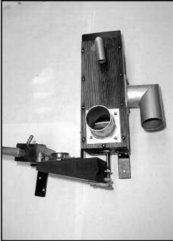
Figure 26. Restored stack vacuum cutout unit.
