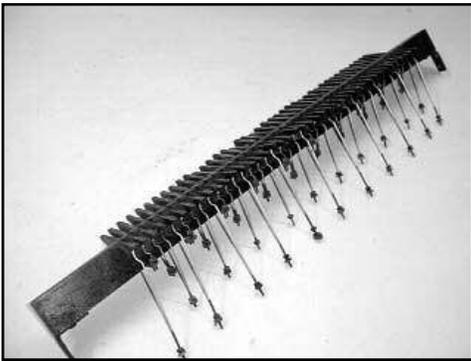
Figure 34. Stack linkage mechanism.
