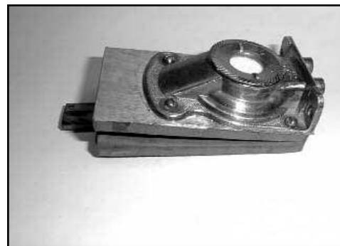
Figure 20. Restored pneumatic valve unit.
