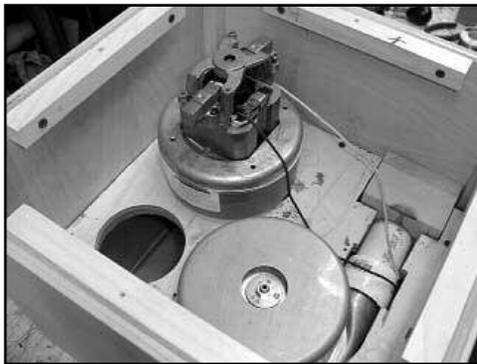
Figure 30. Vacuum Motor pumps.
