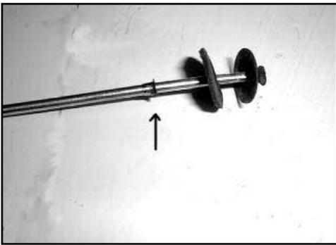
Figure 23. Windchest push rod with facings, the arrow pointing to the collar.
