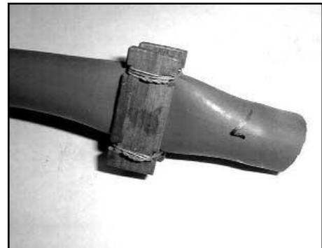
Figure 39. On site emergency repair.
