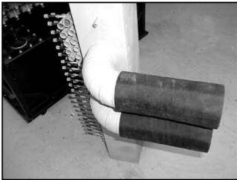
Figure 35. Large wind feeder tubes on wind chest.
