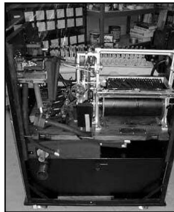
Figure 38. Tracker bar tubing installed.
