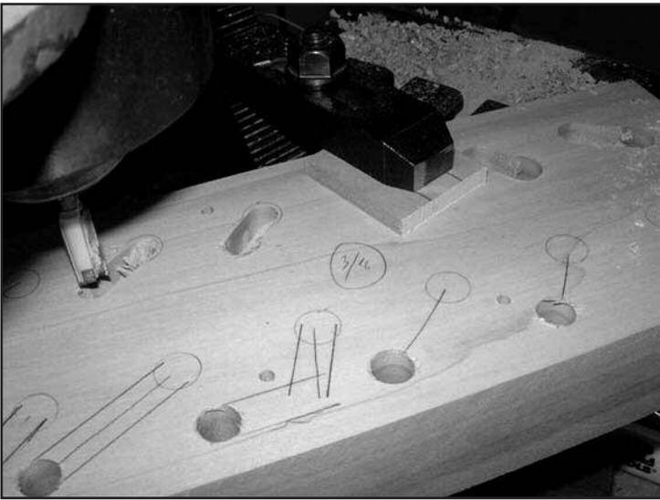
Figure 19. Bottoms of new toe boards are grooved to connect the wind supply to the toe.
