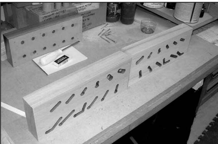
Figure 20. Finished toe board bottom, with all grooves sealed with shellac.
