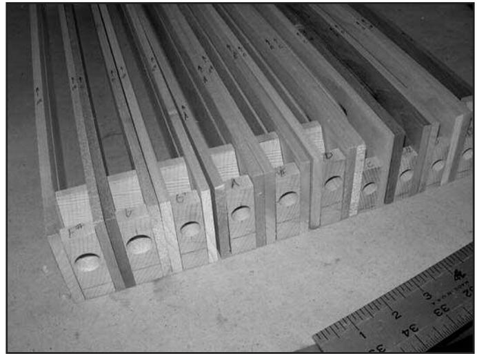
Figure 10. New pipes with sides glued to the block and center divider.
