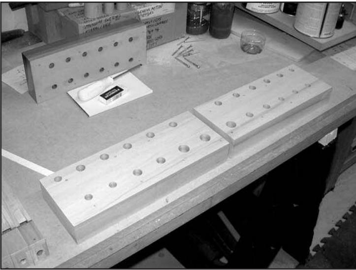
Figure 18. New toe boards to accommodate new pipe spacing.
