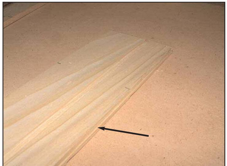
Figure 6. Arrow indicating edge of pipe side with groove for tuner.
