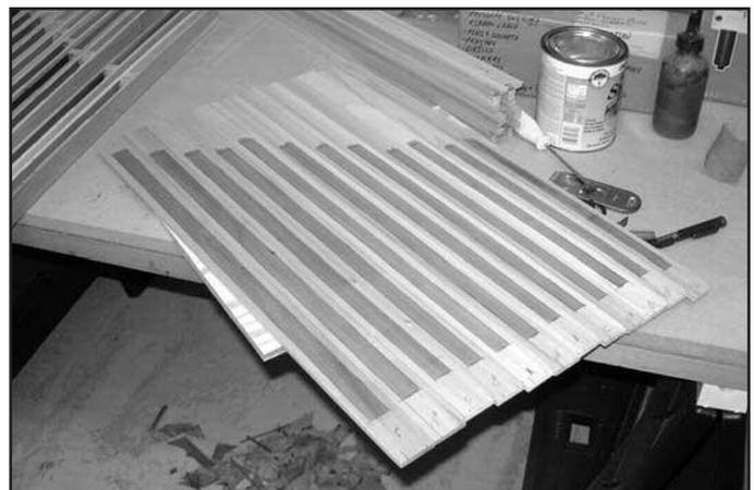
Figure 12. Pipe backs with shellac applied, ready to be glued to side and block assembly.
