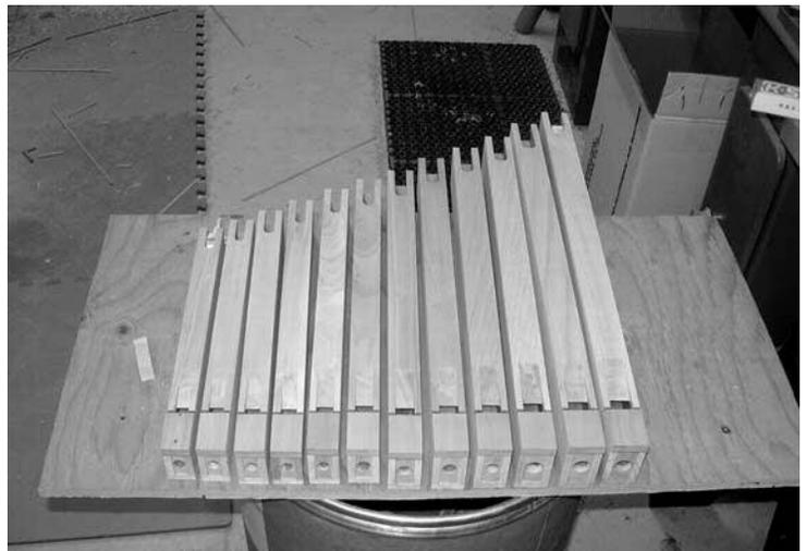
Figure 17. All pipes finished to length, and sides machined flush with the sides.
