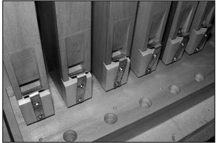
Figure 21. New Haskell violins in place on new toe board.
