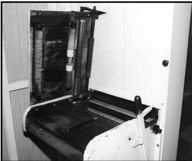
Figure 1. In 1907 the Ruth keyframe connected to a slide that ran across the width of the case. It meant that heavy music crates had to be dragged back from one side to the other. Author’s photograph.
