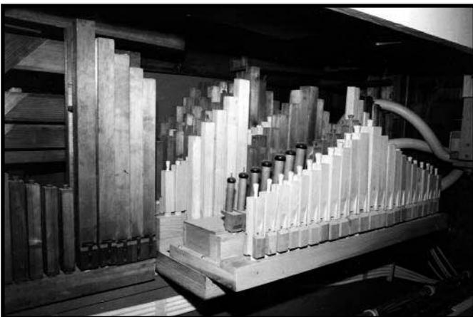
Figure 16. The alternate melody pipework in Ruth organs is typically located behind the violins, on a separate chest. These are the two added voices in the Ohr organ.
