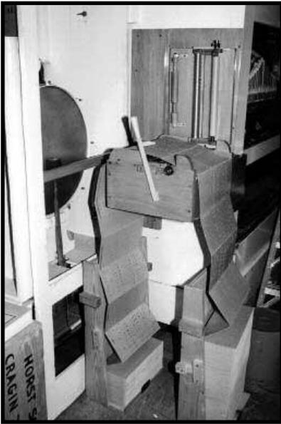
Figure 15. Through the case book systems were not operator friendly. It was a simple matter to change music crates in this style keyframe, which Voigt installed on the rebuilt Ohr instrument.
