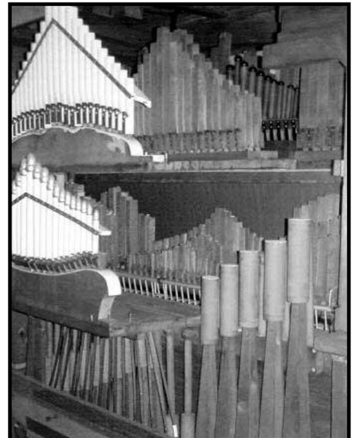
Figure 6. The horizontal channel boards supply wind to the display violins and panflutes, as well as the glockenspiel action. Jim Krughoff photograph.
