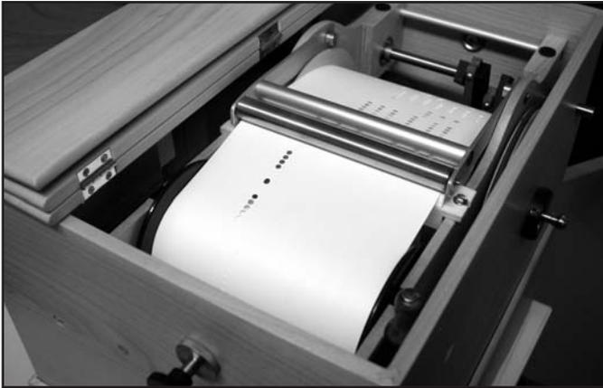
Figure 4. An interior view of the roll frame and pressure bar.
