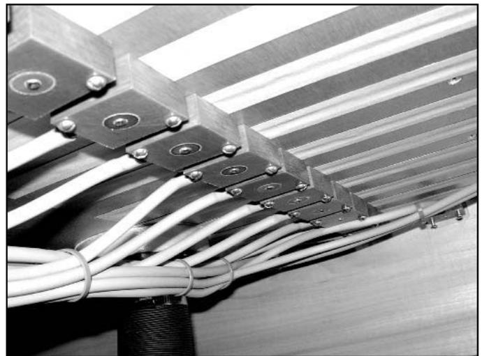
Figure 9. Key action pouch blocks and key action grooves covered with pneumatic cloth.
