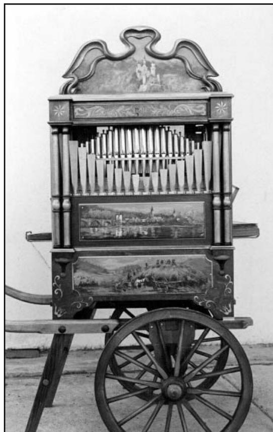
Figure 2. The Maestro organ fitted with trumpets, tin flutes and bourdons. The organ, decorated with Spanish views, is fitted on a neat cart.
