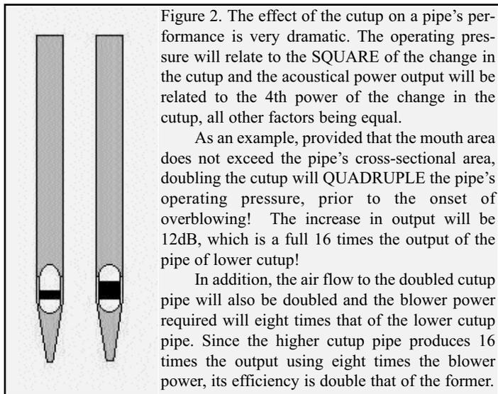
Figure 2. The effect of the cutup on a pipe's performance is very dramatic. The operating pressure will relate to the SQUARE of the change in the cutup and the acoustical power output will be related to the 4th power of the change in the cutup, all other factors being equal.
