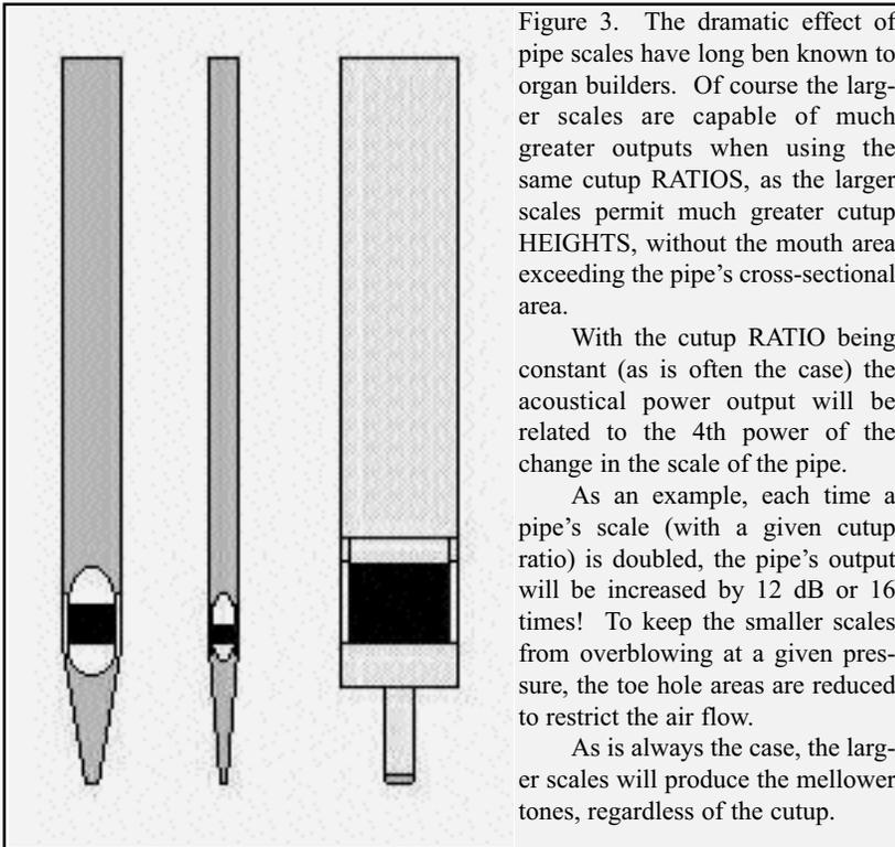
Figure 3. The dramatic effect of pipe scales have long ben known to organ builders. Of course the larg- er scales are capable of much greater outputs when using the same cutup RATIOS, as the larger scales permit much greater cutup HEIGHTS, without the mouth area exceeding the pipe's cross-sectional area.
