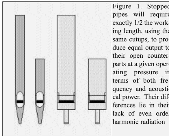
Figure 1. Stopped pipes will require exactly 1/2 the working length, using the same cutups, to produce equal output to their open counterparts at a given operating pressure in terms of both frequency and acoustical power. Their differences lie in their lack of even order harmonic radiation
