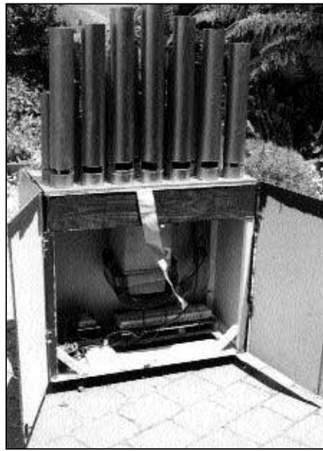
Figure 19. On the lower left is the transformer for the power supply; on the lower right is the pedal board key-switch assembly and in the center is the box housing the blower. All can be seen more clearly in figure 17.
