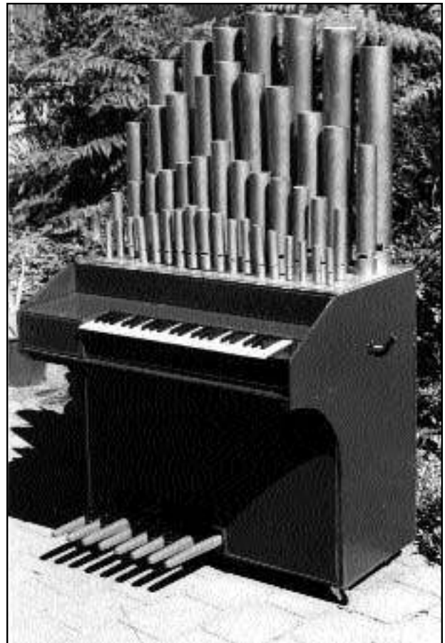
Figure 20. The finished 48-note calliope.
