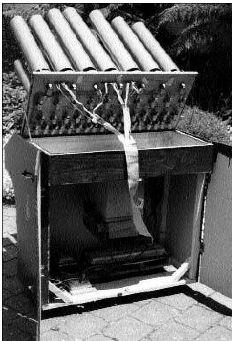
Figure 17. The nearly-finished cabinet revealing the cupboard hinge allowing for easy servicing of the solenoids.
