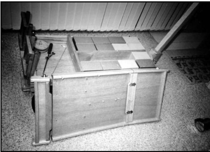
Figure 2. The base of the organ wagon has been modified to accommodate 16 25-note roll boxes.
