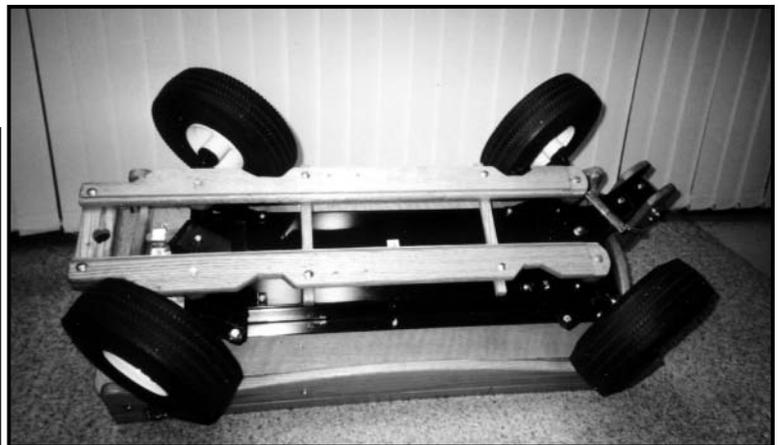
Figure 4. Looking underneath the organ wagon one will find the "skid" rack which also serves as a support for additional storage.
