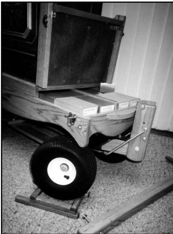
Figure 3. On front of the wagon is the oak boot which makes removing and attaching the handle much easier.
