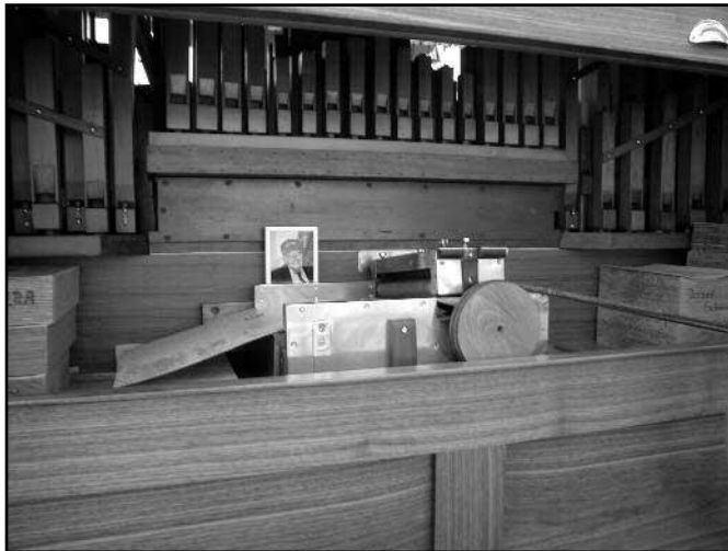
Figure 9. A view of "Jupiter's" key frame and accompaniment pipes (left and right of key frame) and the countermelody bourdon (middle). Photo: Ron Bopp
