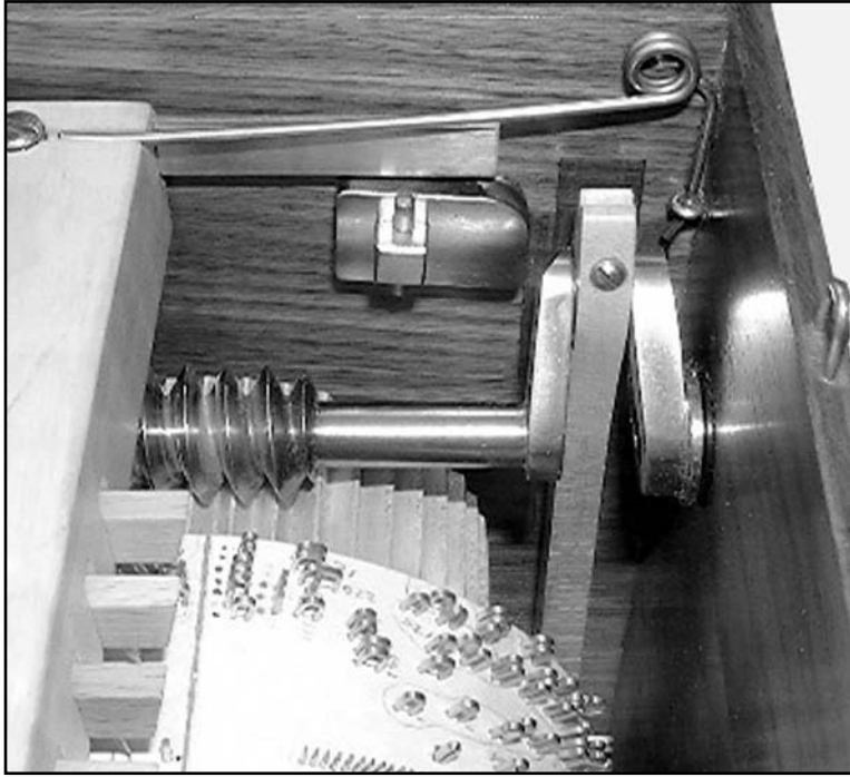
Figure 7 (above). The crank and barrel controls were made from brass and steel.
