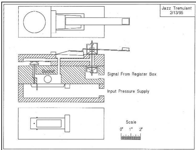
Figure 6. Drawing with a cross section of the tremulant.
