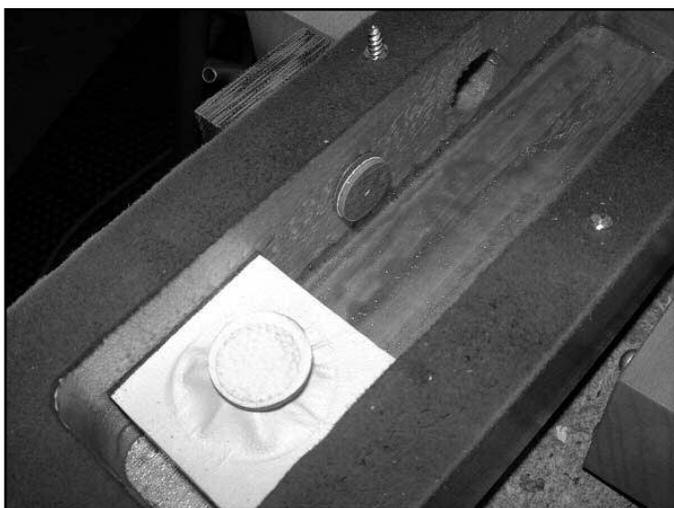
Figure 7. Extra pouch and valve for operation from a vacuum signal.
