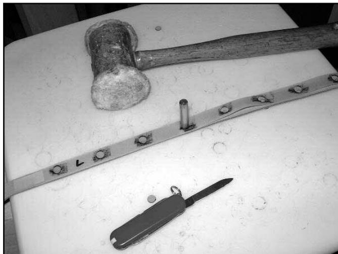
Figure 18. Punching through the paper transfer strip and gasket.
