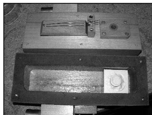
Figure 10. Center and bottom layer of tremulant.
