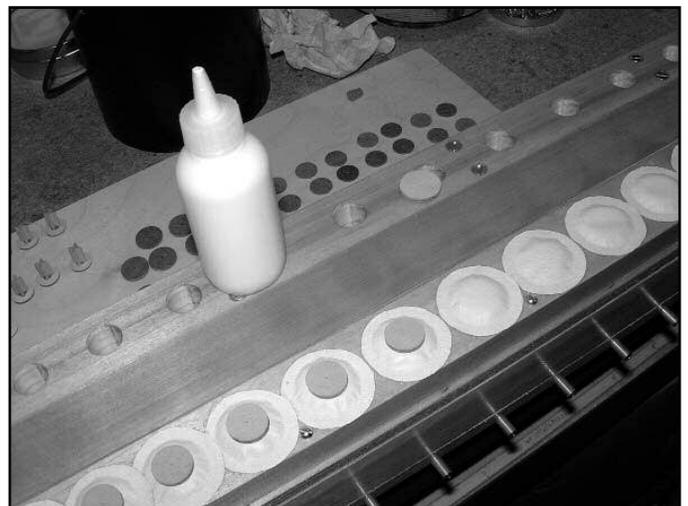
Figure 15. Nearly finished pouch board with some of the lifter disks in place.
