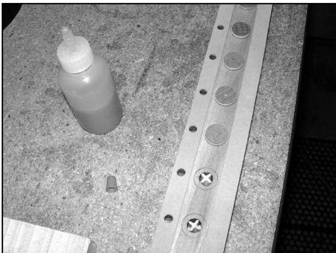
Figure 13. Bottom board of jazz chest with a few valves installed.
