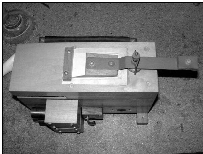
Figure 11. Top view of tremulant showing hinged weighted arm.
