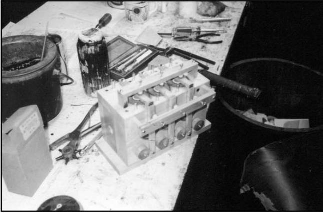
Figure 10. The new register assembly.
