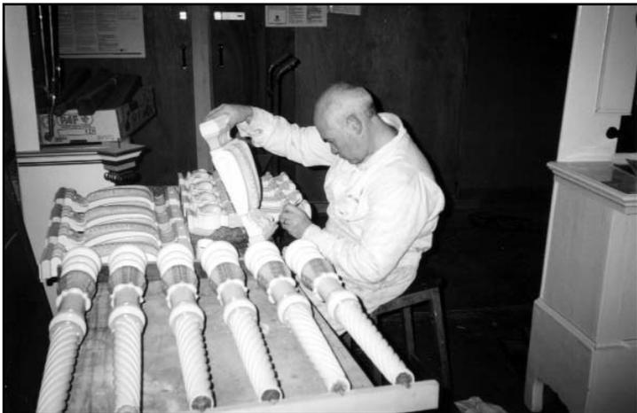
Figure 4. Repainting the facade parts and columns.
