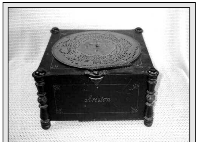
Figure 4. The 24-note Ariston was made by Paul Ehrlich in Leipzig, Germany, and was one of the most successful of the German organettes. From 1885 through the early 1900s hundreds of thousands of these machines were sold. The machine plays a cardboard or metal disc which rotates over the key frame. All the valves are open unless the disc holds them shut. Rod linkage operates the valves from the keys. The machine plays the music as the holes in the disc go over the keyframe opening the reed valves. The music is titled in German, French and English.
