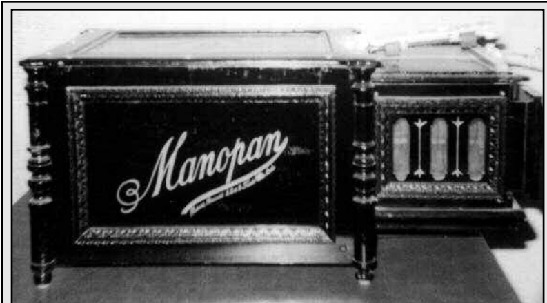
Figure 1. The 39-note double-reeded Manopan was made in Leipzig, Germany by Euphonika Musikwerke from the late 1880s to early 1900s. The organette plays cardboard or metal loops. Each note has two reeds tuned to the same pitch except the four lowest bass notes which are tuned an octave apart. The double reeds produce a full, rich quality music. A 39-note triple-reeded Manopan was also made and is very rare.
