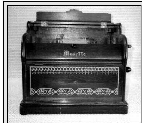
Figure 6. The 16-note Musette was made by the Aeolian Organ and Music Co. of New York in the mid-1880s. The machine has a 16-note tracker bar with 16 small pneumatics which open the pallet valves to the reed chamber. These early pneumatic organettes led to the development of the pneumatic system used in player pianos and other automatic musical machines.
