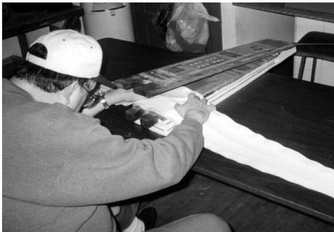
Figure 8. Attaching the leather to the pump boards.
