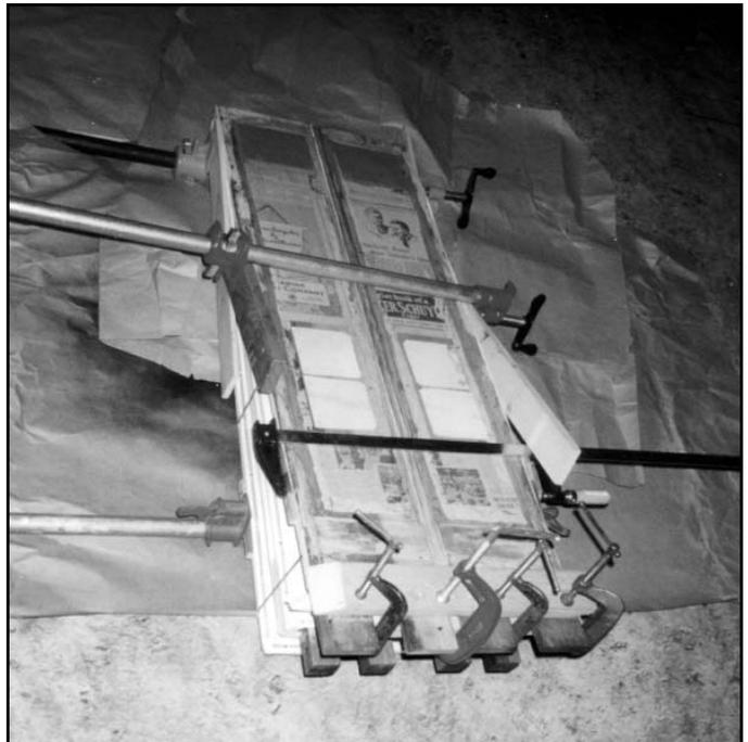
Figure 10. The two pumps being glued back into place.
