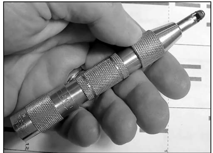
Figure 12. A hand-made, hollowed-out center punch.
