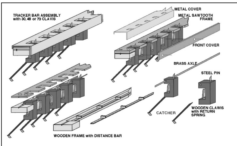
Figure 18. Tracker bar assembly and its components.
