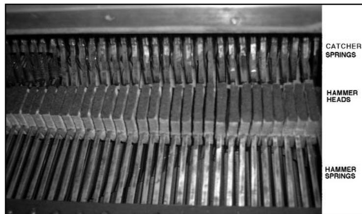
Figure 14. Hammers, hammer springs and stop and go springs of a 48-note Piano Melodico. Collection C.F.C. Greinacher.
