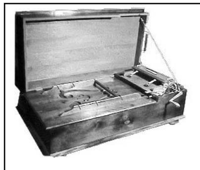
Figure 7. Piano Melodico, similar model as in Figures 5 & 6. During restoration the instrument was altered to manual drive. Collection C.F.C. Greinacher.
