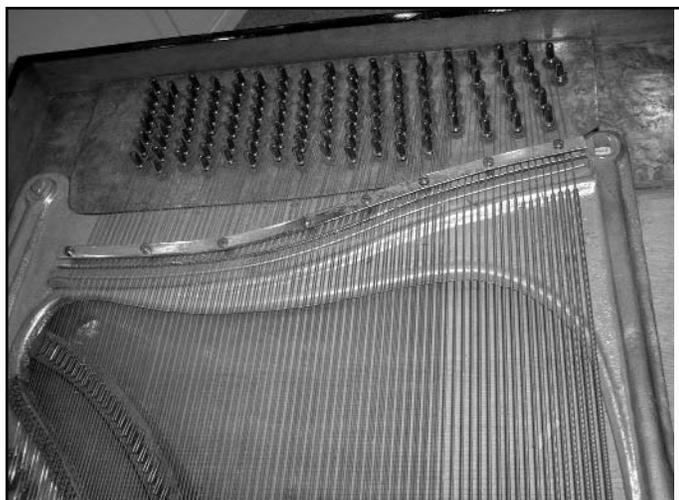
Figure 20. Stringframe, strings and tuning pins of a 73-note Piano Melodico. Collection C.F.C. Greinacher.
