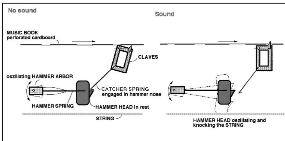
Figure 16. Hammer Control Mechanism of the Piano Melodico.
