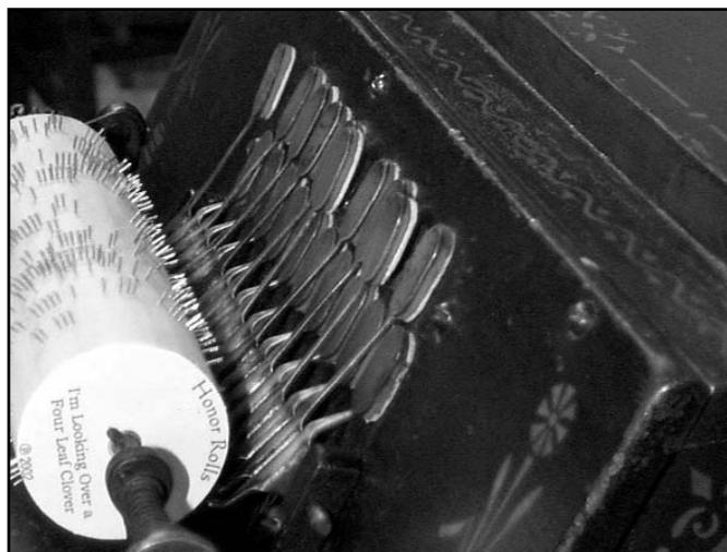
Figure 3. The pins on the roller lift the valves to play the 20-note scale. The roller plays for about 40 seconds in three revolutions and then returns to the beginning.
