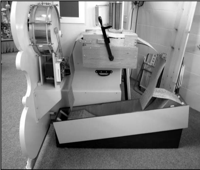
Figure 7. Behind the snare drum wing of the 56-key Wellershaus is the key frame and endless book arrangement.
