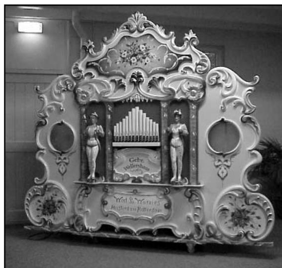
Figure 6. The 52-key Wellershaus was originally a barrel organ but later converted to the 56-keyless book system.
