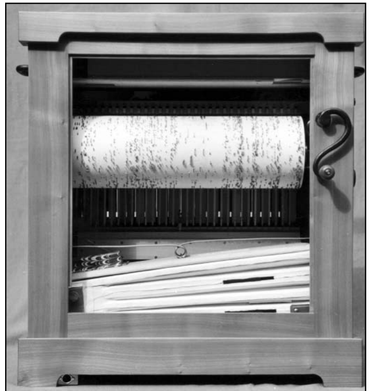
Figure 4. The back side of the Fairy-tale organ case reveals the bellows and reservoir at the bottom and the pin-barrel at the upper middle portion of the case. Note the artistic crank handle.
