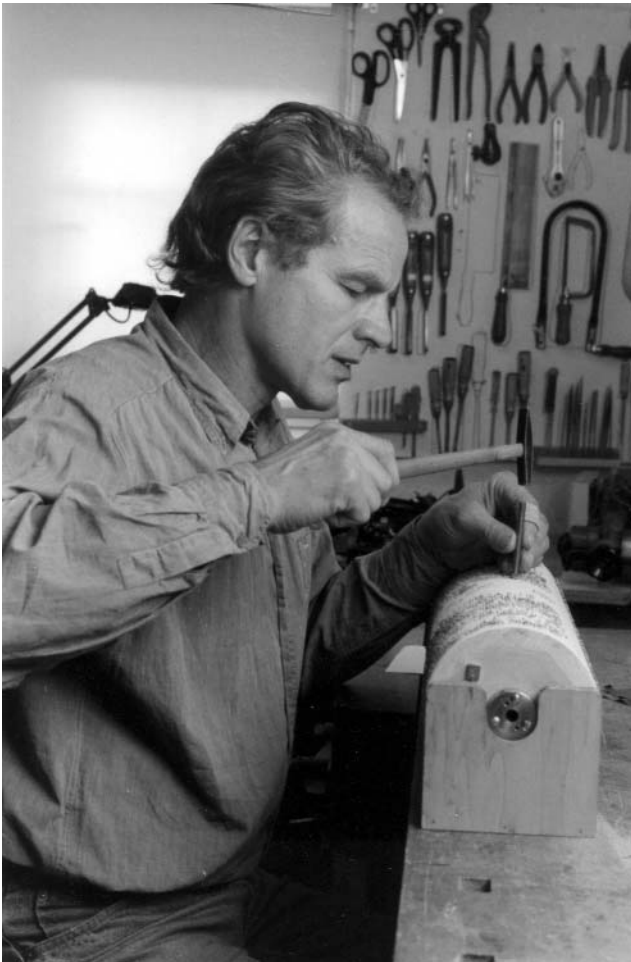
Figure 14. Hansjörg Leible pinning a barrel for a Fairy-tale organ.
